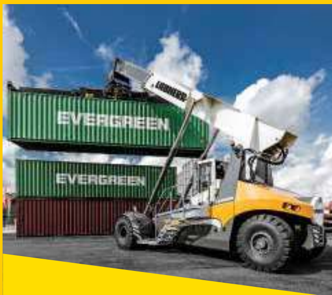
Liebherr Reachstacker LRS 545 hardworking handling container at Antwerp Port
