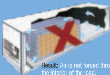
Load placed in the front of the container
