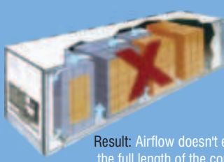
Excessive space between the load
