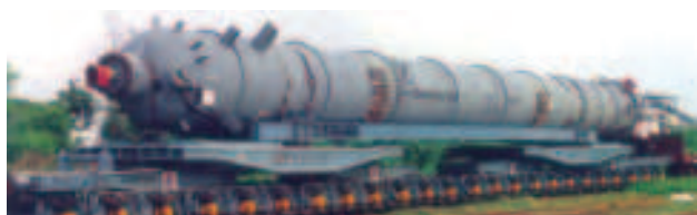
Project cargo: ACTL's 24-axle heavy duty wagon can carry 350 MT of single package for thermal and power projects in the country.
