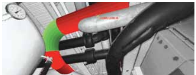
Clash highlighting between a proposed new pipe run and as-built laser scan data.
