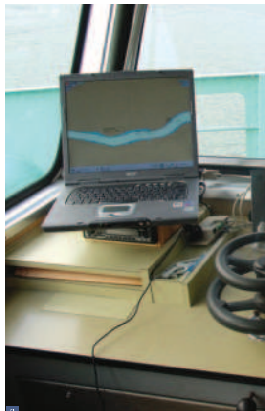
3 An Electronic Chart Display and Information System (ECDIS) displays the information from electronic navigational charts (ENC) and integrates position information from the Global Positioning System (GPS) and other navigational sensors, such as radar and automatic identification systems (AIS). It may also display additional navigation-related information, such as Sailing Directions and fathometer.
