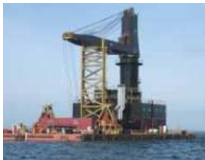
The K50 crane offers a capacity of 50-tonnes in grab operation and an outreach of 32m
