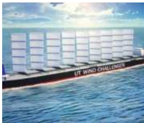
THE DEPICTION OF A CARGO SHIP EQUIPPED WITH THE WIND CHALLENGER PROJECT SYSTEM OF SAILS
