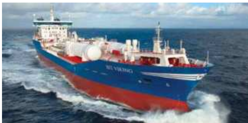
The world's first LNG-fueled product tanker, the Bit Viking , is now officially in service. The 25,000-dwt product tanker underwent an LNG main machinery conversion. The vessel is now also the largest commercial vessel to use LNG as fuel. During the conversion, the vessel's main engines were rebuilt for dual-fuel operation, and two 500-cubic metre LNG tanks were placed on deck, giving the vessel a range under LNG of 12 days. However, such conversion may not be feasible for many ships due to limited engine retrofit options and lack of space for LNG tanks.
